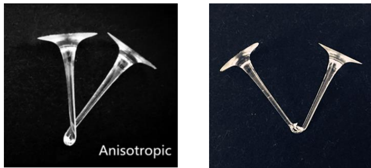
Figure 1: flexible polystyrene (left) and cracks when trying to recover the sample (right)
