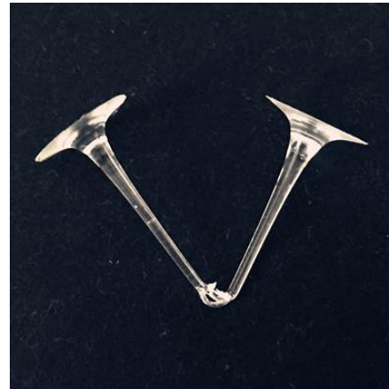
Cracks when trying to recover the sample after bending
